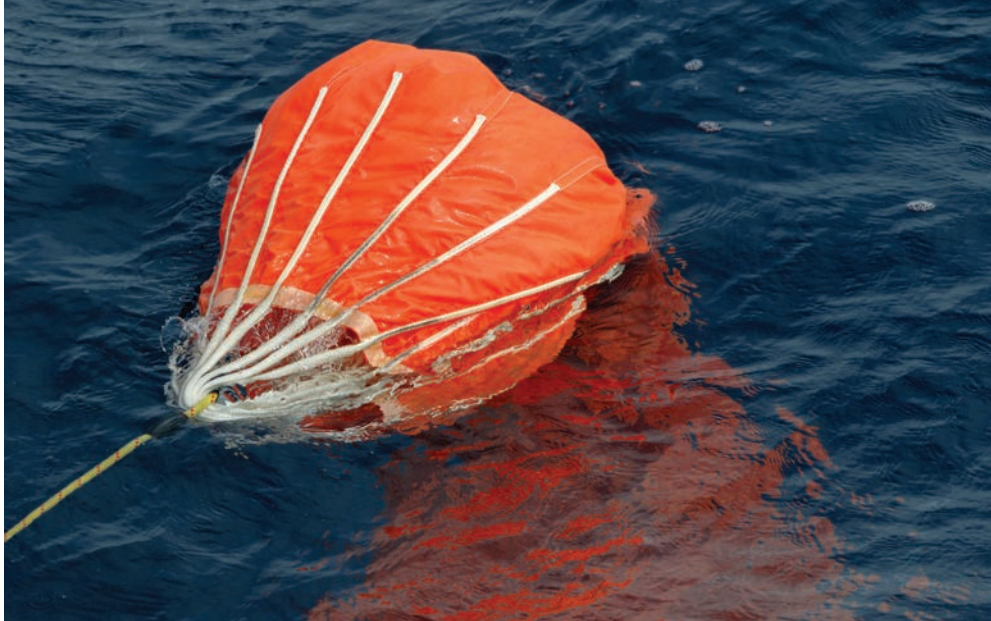
Modern sea anchor (drogue). Photo by Ed Dunens (Wikimedia Commons, CC BY 2.0).
